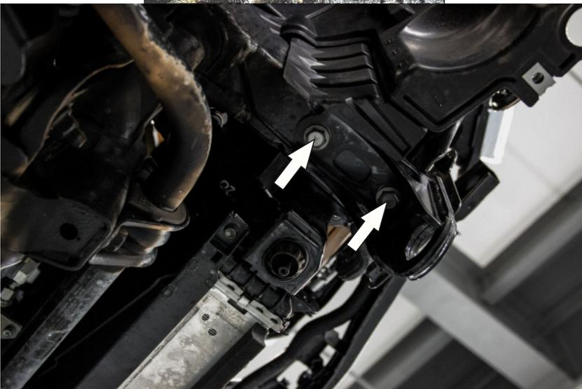
20. Unscrew 2 tension bolts of standard
