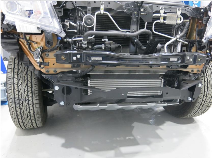
25. Install the winch bracket (pos. 1) onto the vehicle. Secure to adapters and frame boosters using bolts M12x30 (pos. 9), nuts M12 (pos. 11) and washers (pos. 12). Adjust the winch bracket. Tighten all screw joints, including adapters and frame boosters.
