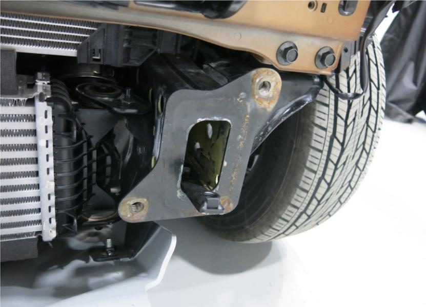
21. Insert embedded part M12 (pos. 8) into the frame on the left.
