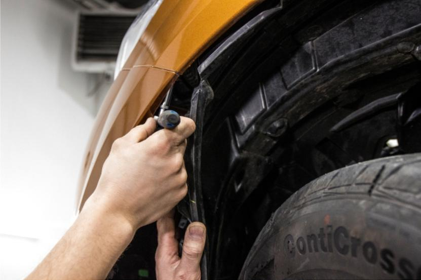
12. Carefully unbend plastic wheel arch covers on the vehicle's left and right, and unscrew self-tapping screws of the bumper clamp.
