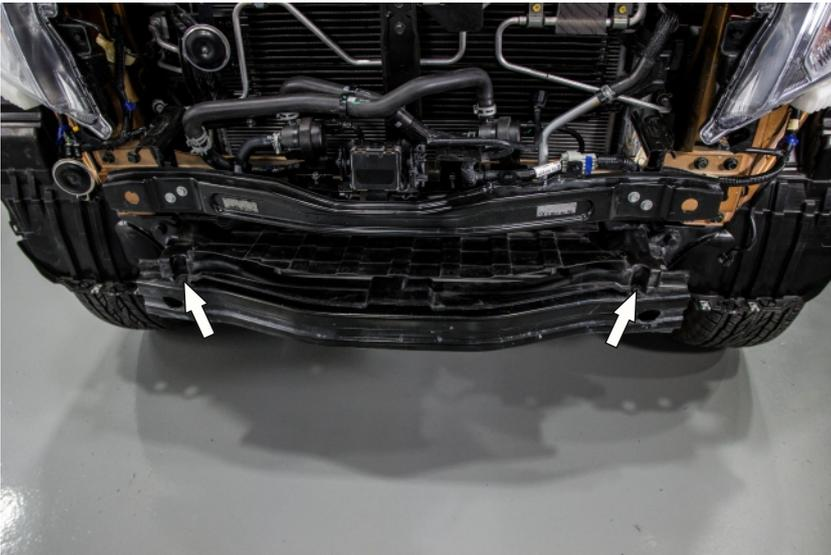
18. Remove the air intake clips.
