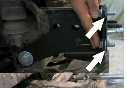
17. Place bolts M10x30 (17) with washers M10x30 (30). Push support bracket to the front of the chassis. If there is a gap of more than 2mm, place washers M10x30 inside.
