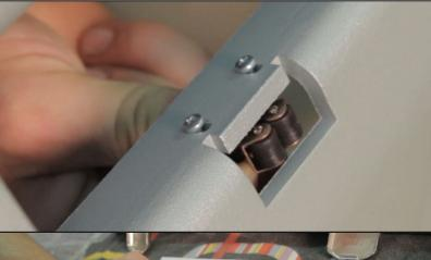
23. Mount roll latches (32) to bumper (1) with screws M3x12 (20) and nuts M3 (24).
