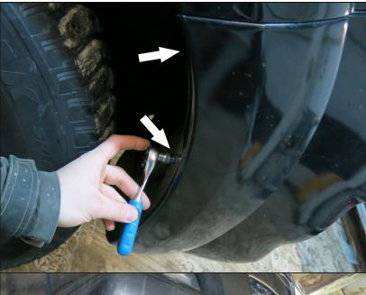
4. Remove lower bumper retaining screws and scrivets.
