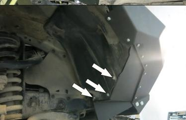
40. Mark drill points on plastic fenders in accordance with the apertures in the flaps. Using a 6-7 mm drill bit, drill holes.
