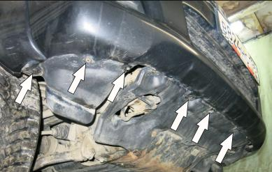
5. Remove lower bumper retaining screws.
