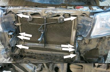
10. Remove plastic scrivets and remove plastic side deflectors.
