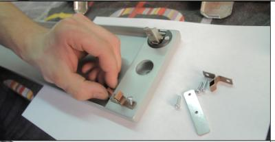
24. Mount opposite latch to license plate holder (5) with screws M3x12 (20) and insert nut (10).
