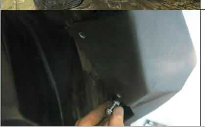
37. Using a 6-7 mm drill bit drill holes in plastic fender in accordance with holes in flap. Fix flaps with bolts M6x20 (22), washers M6x12 (27) and nuts M6 (33).
