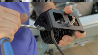
32. \* Mount LED lights into brackets (6). Adjust and tighten them.
