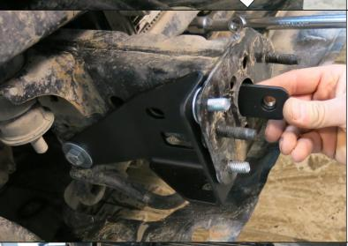
18. Place insert nut 2xM12 (9) inside of the chassis. Screw on bolts M12x30 (19) with washers M12x37 (31).
