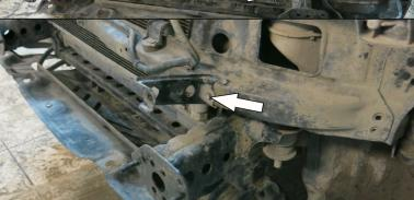
11. Remove M6 bolts. Remove side brackets.
