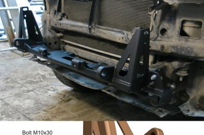
19. Mount winch bracket (2). Use OE bolts and supplied bolts M10x30 (17), bolts M10x25 (16), washers M10x20 (29), washers M10x30 (30) and nuts M10 (26) from the fitting kit bag.
