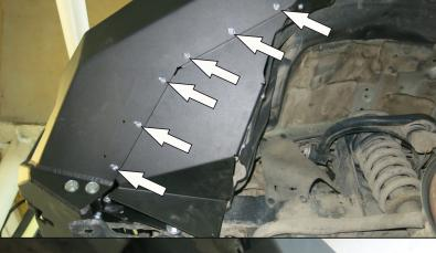
39. Install the flaps using bolts M6x20 (22) and washers M6x12 (27).
