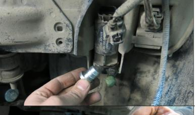
15. Disconnect washer fluid bottle. Remove the pump and insert the supplied plug (13) instead.
