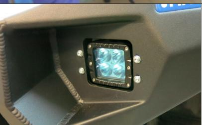
33. \*Install brackets with LED lights using bolts M6x16 (21) and washers M6x12 (27). Adjust the LED position.
