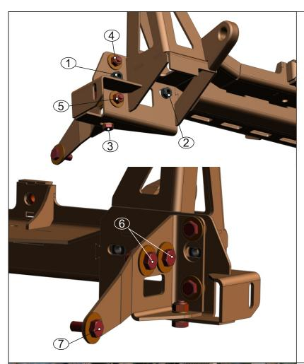
20. Align winch bracket horizontally and vertically.
