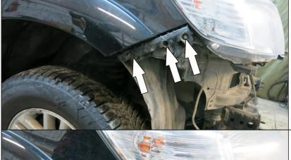
13. Remove M6 bolts and scrivets. Remove plastic side fittings.
