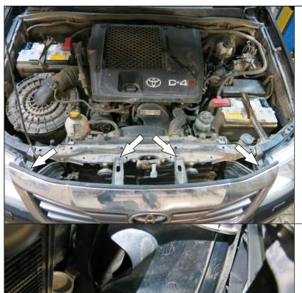
1. Open the bonnet and remove all scrivets holding the grill in place.
