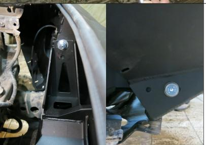
29. Adjust bumper so that there is an equal gap between the bumper and the vehicle body on both sides.
