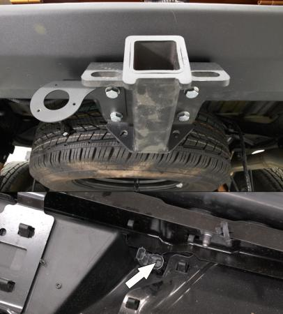
25. Mount tow bar bracket (3) on vehicle using bolts M12x1,25x40 (B) and washers 12 (G). Tighten all screws.
