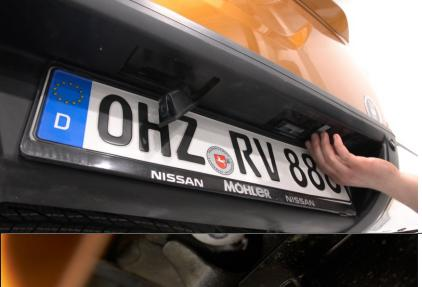
5. Remove license plate lights. Gently pull lights down, turn wire and light for a 90 degrees.
