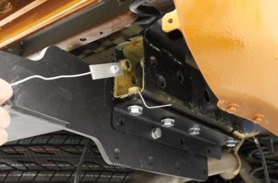
13. Mount inside nut M10(I) into the vehicle frame from the right side.
