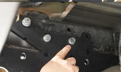
15. Mount bracket (2) from left side of vehicle into OE hole using bolt M12x1,25x40(B) and washer 12 (G). Do not tighten yet.
