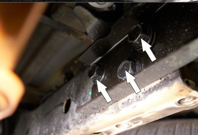
6. Unscrew 3 bolts of rear bumper mount from left and right side.
