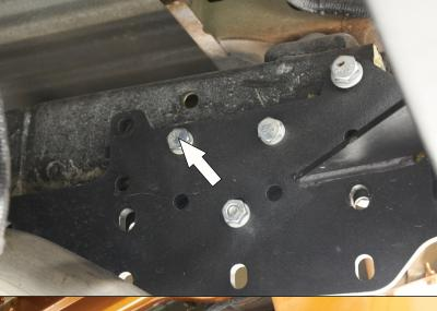
12. Mount bracket (2) on inside nut M10 (I) using bolt M10x40 (10) and washer 10 (F). Do not tighten yet.
