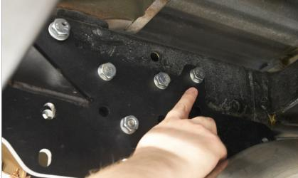
16. Mount inside nut M10(I) into the vehicle frame from the left side.
