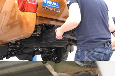
10 . Mount bracket (2) on OE holes in frame using bolts M12x1,25x40 (B) and washers 12 (G). Do not tighten yet.
