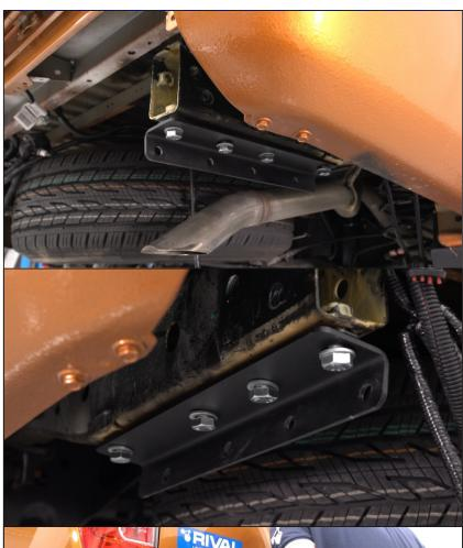
9. Mount reinforcements (5, 6) on vehicle frame from left and right side using bolts M12x1,25x40 (B) and washers 12 (G). Do not tighten yet.
