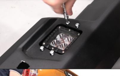
20. \* Mount brackets on bumper body (1) using screw M6x20(C). \* For package with LED lights.
