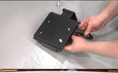
24. Mount socket bracket (M) on tow bar bracket (3).
