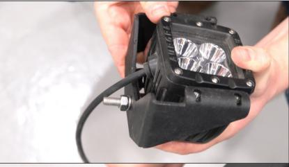
19. \*Mount lights on brackets (4) using fittings from light set. \*For package with LED lights.
