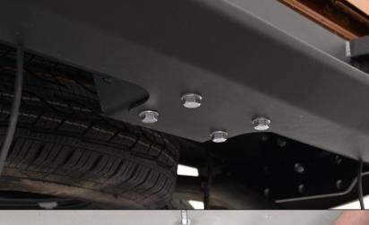
23. \*Mount bumper body (1) on bracket (2) in lower part using bolts M12x1,25x40(B) and washers 12(G) Tighten all screws.
