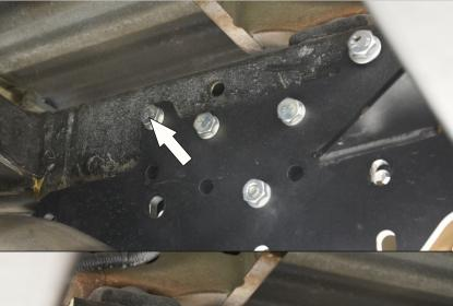
14. Mount bracket (2) on inside nut M10 (I) using bolt M10x40 (A) and washer 10 (F). Do not tighten yet.
