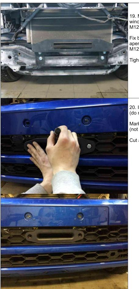
19. Mount brackets #2 and #3 to the winch bracket using bolts M12x30 , nuts M12 and washers #11.
