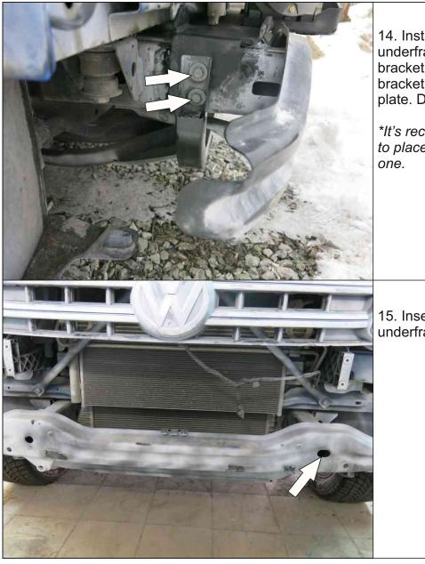
14. Install the winch bracket to underframe. On right side, place winch bracket under the original skid plate bracket. Slightly screw OE bolts of skid plate. DO NOT TIGHTEN YET.
