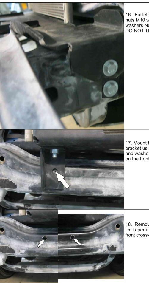
16. Fix left side of the bracket to insert nuts M10 with bolts M10x50 and washers No. 10. DO NOT TIGHTEN YET.
