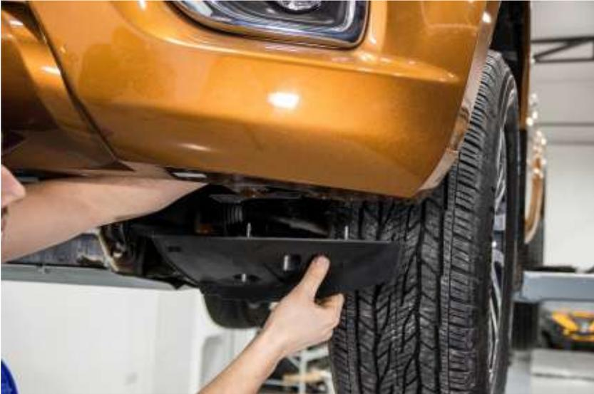
11. From the bumper inside, screw out 2 nuts which fasten the bumper skirt lateral part, and dismount the bumper skirt lateral part.
