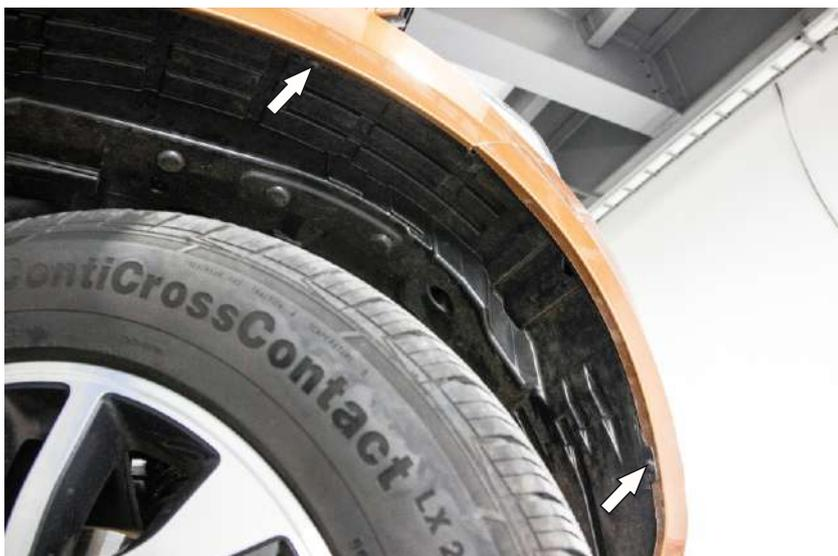
8. Screw out self-attack screws fastening the bumper in arches on left and right, two on each side.
