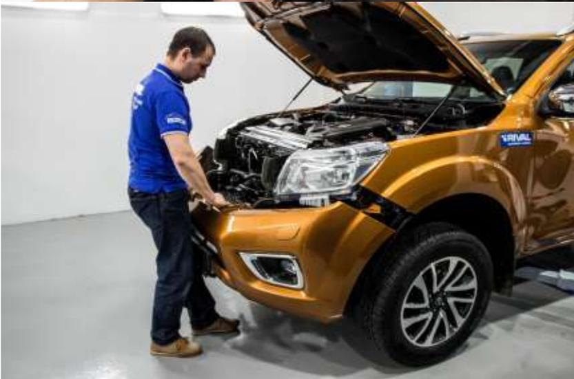
13. Dismount the bumper. Pull the bumper edge with snapping off snaps, moving from the bumper margin to the centre.
