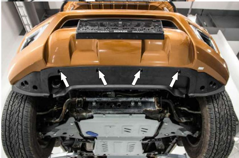
9. Screw out 4 bolts which fasten the bumper skirt central part. Remove the bumper skirt central part.
