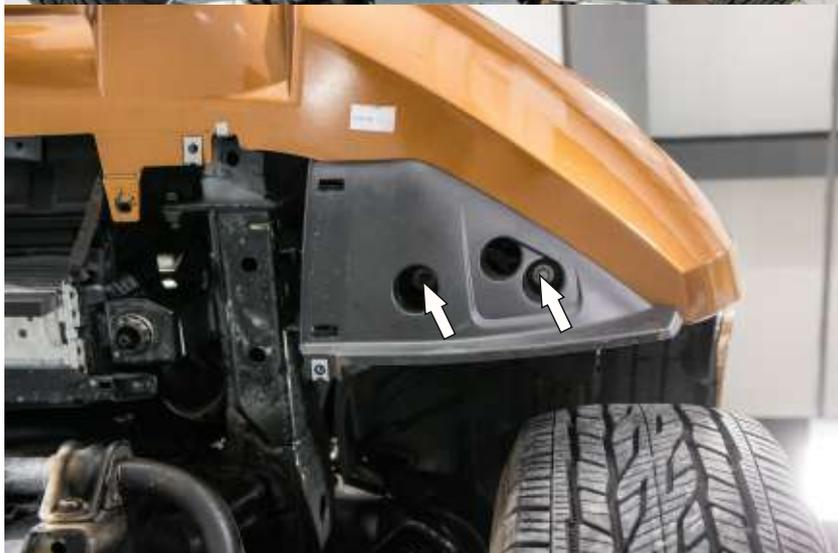
10. Screw out bolts fastening the lateral part of bumper skirt on the car left and right sides, two on each side.
