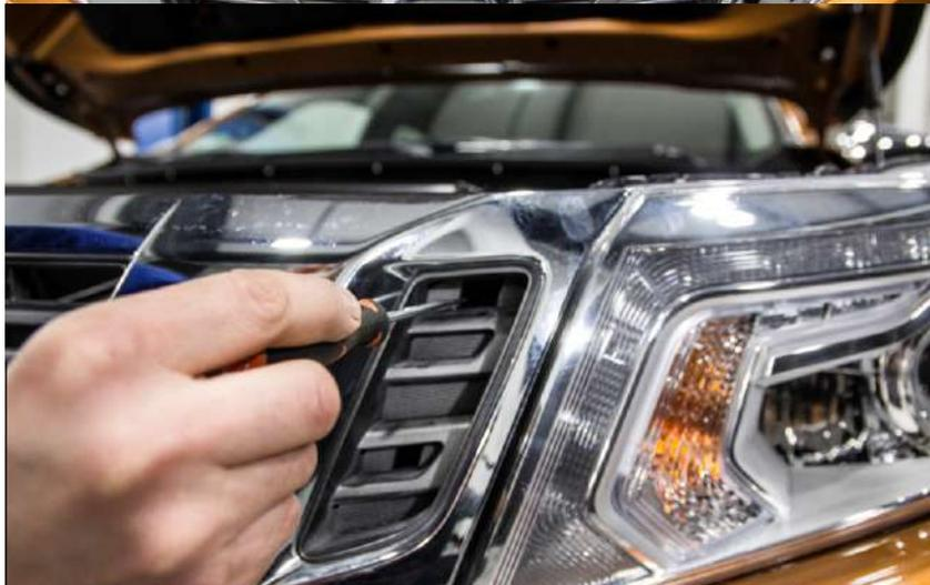
4. Near headlamps, remove clips of radiator grille on left and right.
