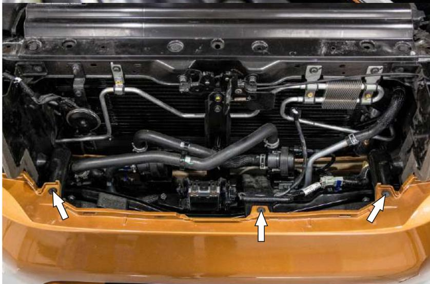
7. Remove clips which fasten the bumper.
