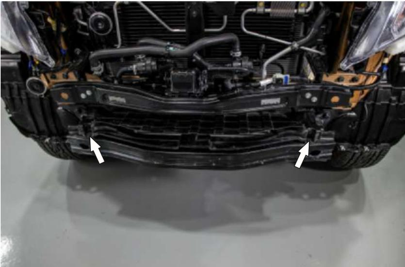
18. Remove clips which fasten the air intake. Dismount the air intake.
