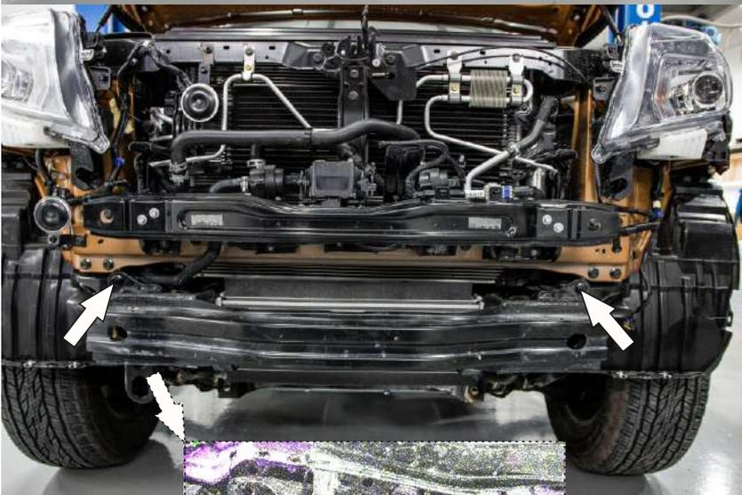
19. Screw out 4 bolts of the frame stiffener fastening. Dismount the stiffener.
