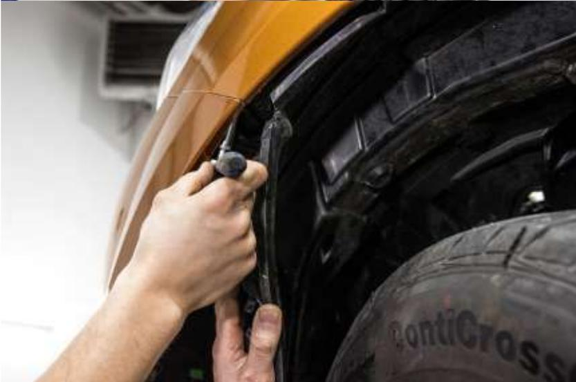
12. Carefully bend out plastic underwing flaps on the left and right sides of the car, and screw out self-attack screws which fasten the bumper.
