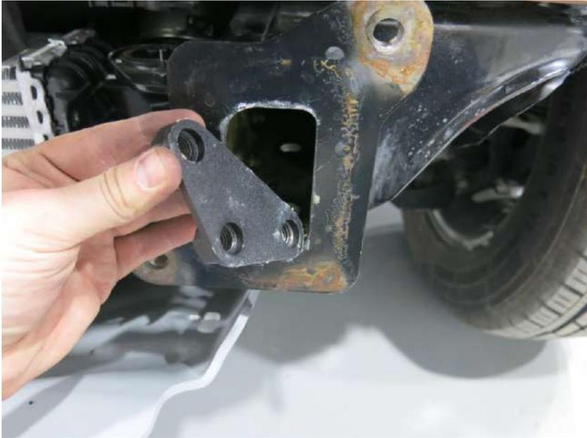
21. Insert captive pins 3xM12 (item.3) into the car frame on left and right.
