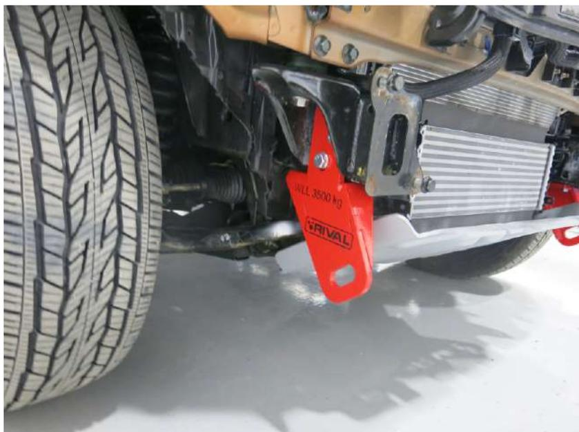
25. Fasten the towing loop (item 2) in lower part with standard bolts which fasten the towing eye.
