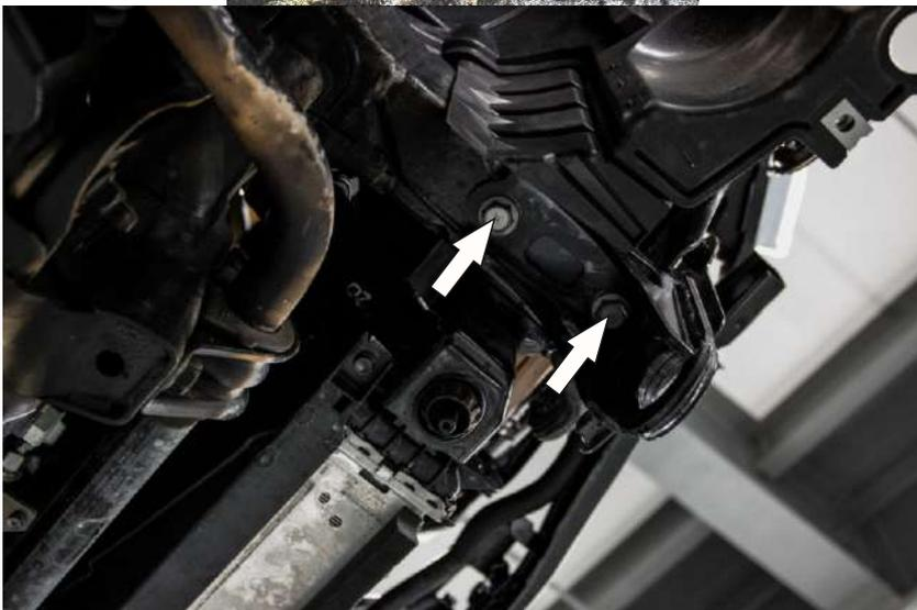
20. Screw out 2 bolts which fasten the standard towing eye. Dismount the towing eye.
