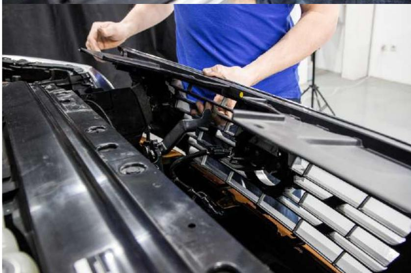
6. Carefully dismount the radiator grille by snapping off snaps in the lower part.
