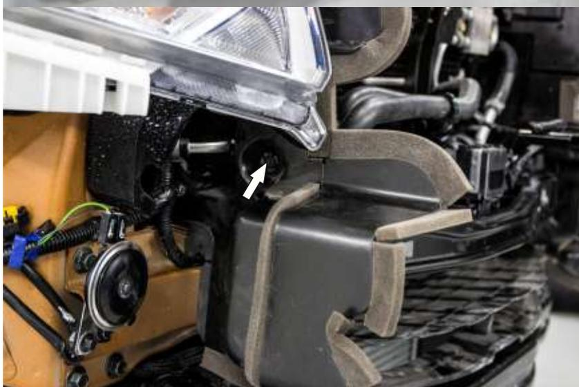
16. Remove clips fastening the plastic dust caps.
