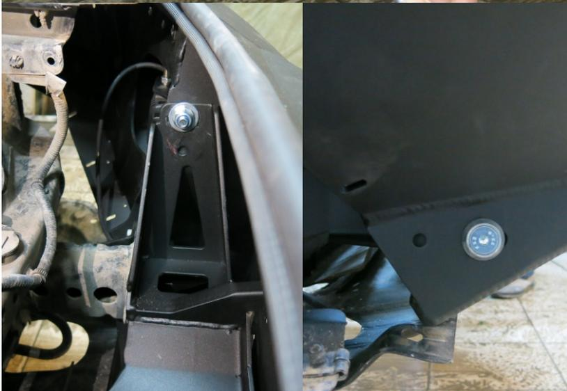
27. Adjust bumper (1) so that there is an equal gap between the bumper and the vehicle body on both sides.
