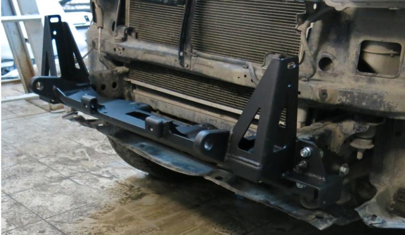
19. Mount winch bracket (2). Use OE bolts and supplied bolts M10x30 (B), washers M10 (K), washers penny M10 (M) and nuts M10 (I) from the fitting kit bag.
