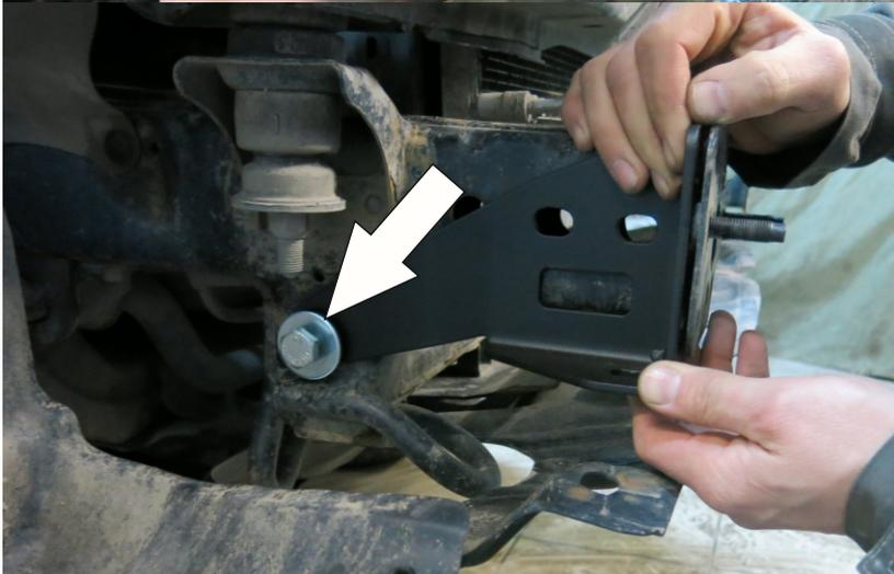
16. Mount support bracket (3) and fix it with bolt M12x30x1,25 (C) with washer penny M12 (N).
