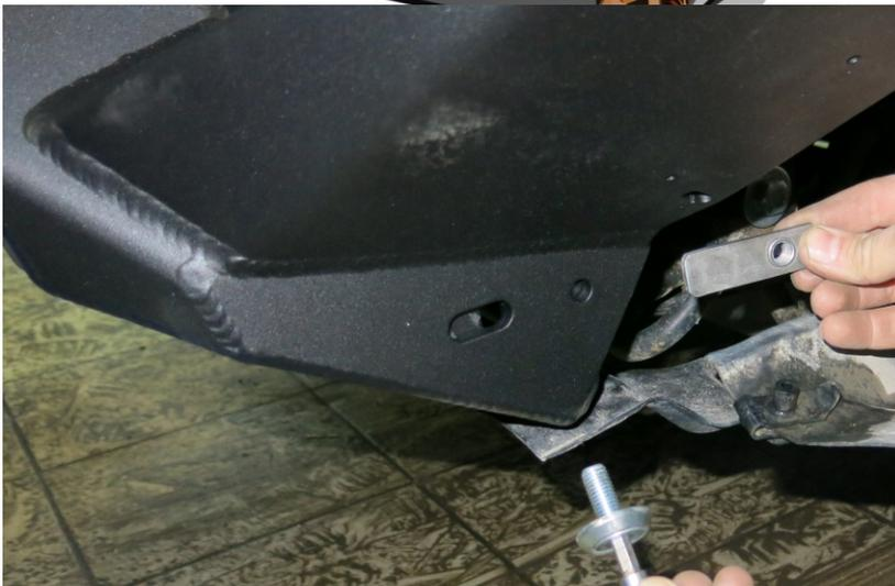
26. Place insert nut plate M10 (O) as shown. Screw blind-head bolt M10x30 (F) with countersunk washer (Q).
