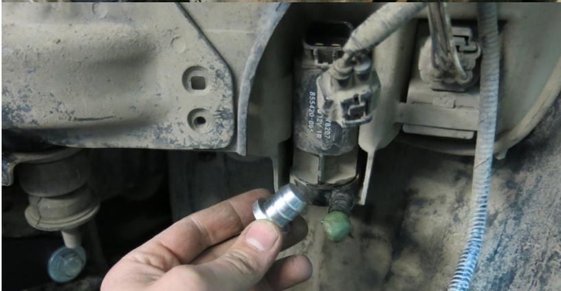
15. Disconnect washer fluid bottle. Remove the pump and insert the supplied plug (P) instead.
