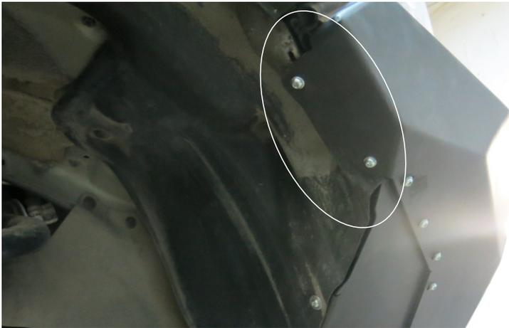
24. Install bumper body (1) onto the vehicle, make sure the plastic fender goes inside.
