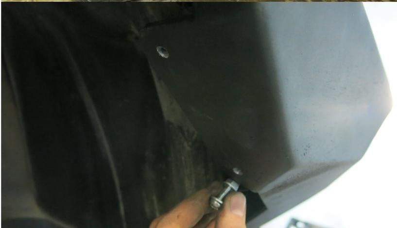
34. Using a 6-7 mm drill bit drill holes in plastic fender in accordance with holes in flap. Fix flaps with bolts M6x20 (A), washers M6 (J) and nuts M6 (H).
