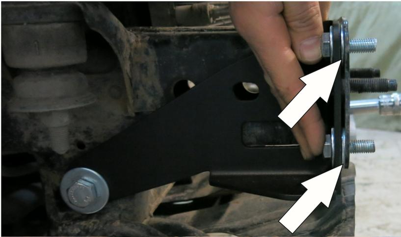
17. Place bolts M10x30 (B) with washers penny M10 (M). Push support bracket to the front of the chassis. If there is a gap of more than 2mm, place washers penny M10 (M) inside.
