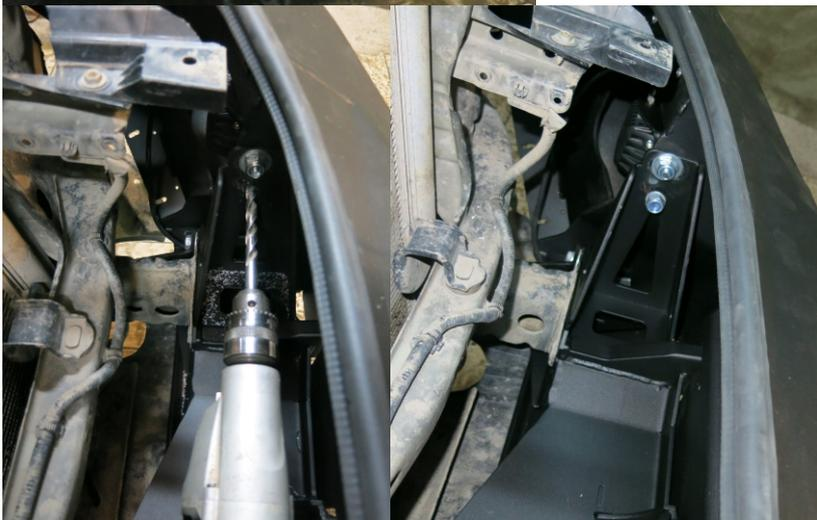
29. Using a 10mm drill bit, drill into the hole through the existing hole of the winch bracket (2) from both left and right. This is to increase the size of the existing hole.
