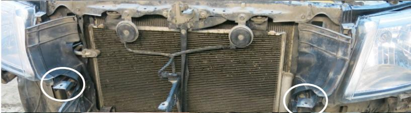
39. Cut plastic brackets as shown so the brackets supplied for radiator grill (T, U) can be installed.
