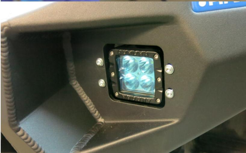
31. \*Install brackets (6) with LED lights (9) using bolts M6x20 (A) and washers M6 (J). Adjust the LED position.
