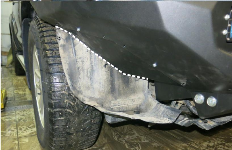
33. Install flaps (7, 8) as shown using the bolts M6x20 (A) and washers M6 (J) supplied.
