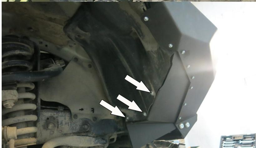
37. Mark drill points on plastic fenders in accordance with the apertures in the flaps (7, 8). Using a 6-7 mm drill bit, drill holes.
