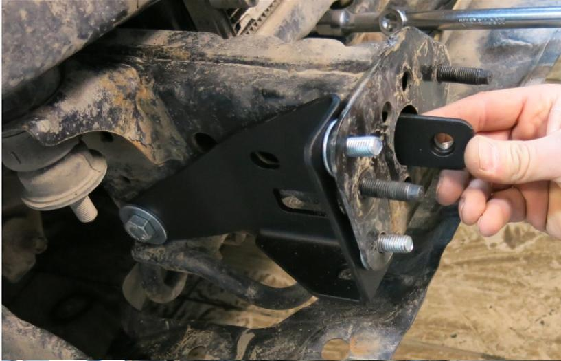
18. Place insert nut 2xM12 (R) inside of the chassis. Screw on bolts M12x30 (D) with washers penny M12 (N).
