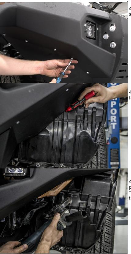
47. Mount flaps (8) on bumper using screws M6x20(D) and washers 6 (J).
