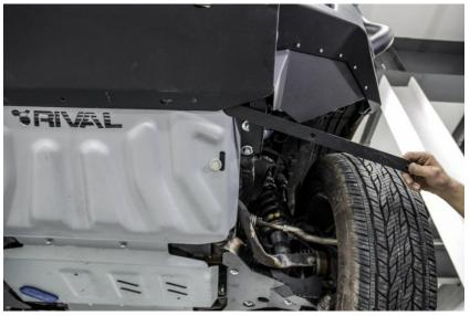
53. \*Fix underbody armour to the bumper body using insude nuts (Q), screws M10x30 (E) and inside washers (N).
