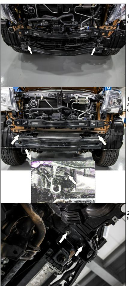
18. Remove caps of air intake mount. Remove air intake.
