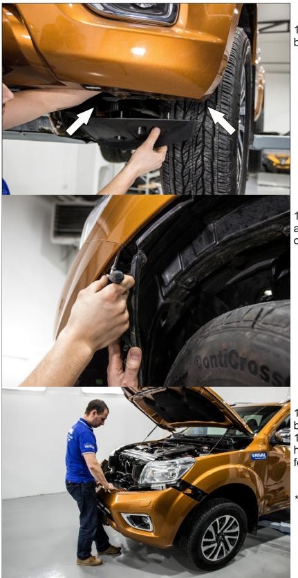
11. Remove 2 nuts from inside of the bumper. Remove side part of the lip.
