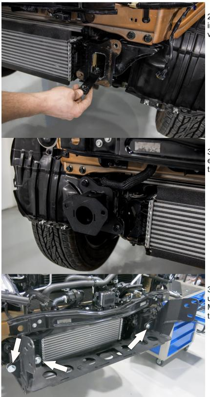
29. Mount inside nut M12x1,25 (R) into the chassis from the left side of vehicle.
