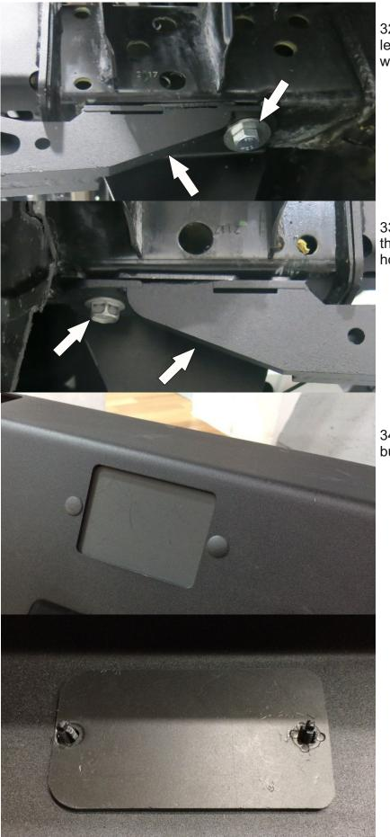
32. Mount lower part of bracket from the left side using bolts M12x1,25x40 (C) and washers 12 (L).
