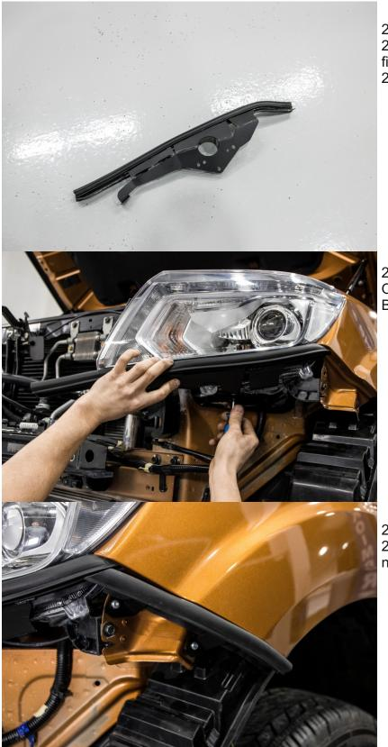
24.Cut seals (9) on parts with lengh t 260mm and 490mm for left and right fide of vehicle.
