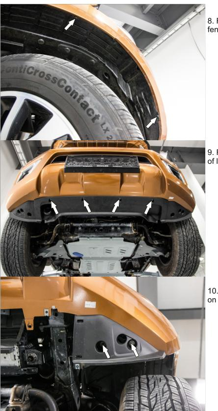
8. Remove 2 screws from inside of the fenders on each side of the vehicle.
