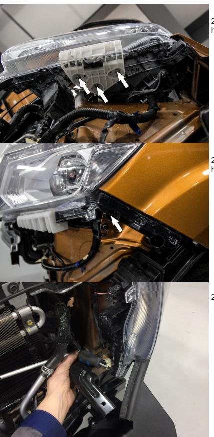
21. Remove screws. Remove plastic holders.
