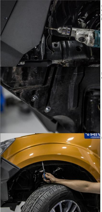
50. Mark a hole from inner side of the wheel fender from both left and right side of vehicle. Drill a 6 mm diameter hole.
