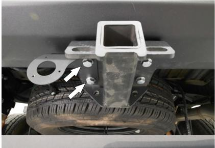
11. Fix the tow bar (3) on the left side, through the socket bracket (L).
