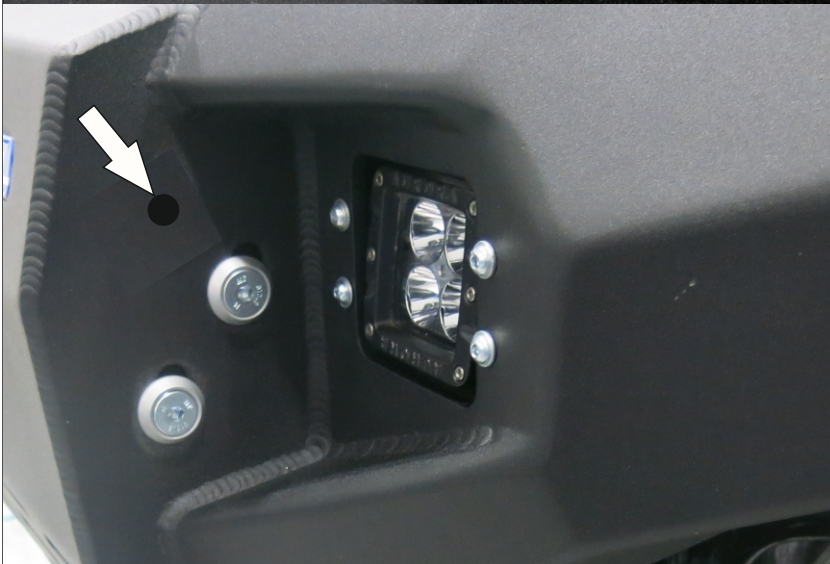
43. Drill 10mm holes in winch bracket through the holes in bumper.
