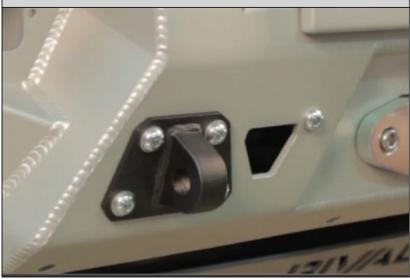
32. Mount towing hooks (8). Tighten M10x30 round-head screws (29).
