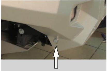
27. Place bumper body to the winch bracket using M10x30 countersunkhead screws (28), countersunk washers (19), M10x30 washers (37) and M10 nuts (32). DO NOT TIGHTEN YET.
