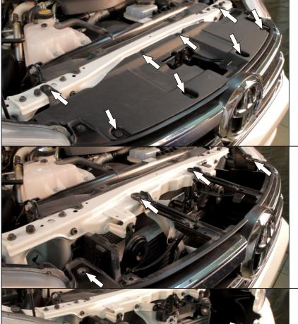
1. Open the bonnet and remove all scrivets holding the grille in place.
