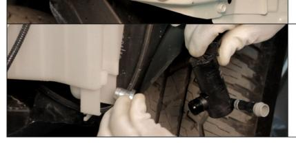
14. Disconnect washer fluid bottle, remove the pump and insert the supplied plug instead (18).
