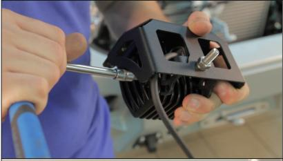
33. LED lights have been mounted to the Bumper Body for transport purposes and are not tightened to the specified tension.
