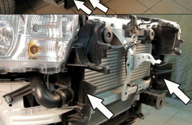
10. Remove 4xM10 bolts fixing crash beam to chassis. Set aside for re-use later on.
