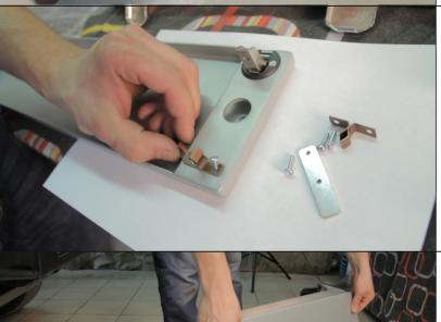
21. Mount opposite latch to license plate using M3 nut plate (14) and screws M3x12 (25).
