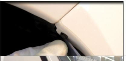
5. Remove all scrivets retaining bumper along inside edge of wheel arches.
