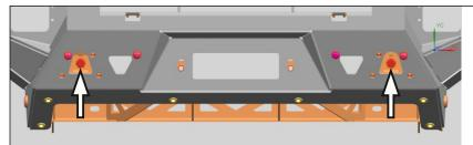
26. Give a few turns to M12x30 bolts (24) with M12x24 washers (38) which will assist with seating.
