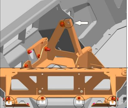
30. Using a 10mm drill bit drill a hole through the existing hole of the winch bracket from both left and right.
