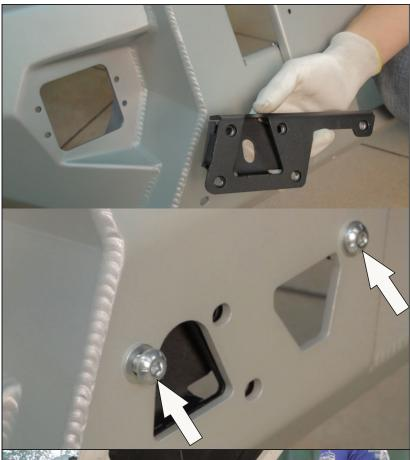
23. Mount adapters (3, 4) to bumper using round-head screws M10x30. Use 2 screws from each side.
