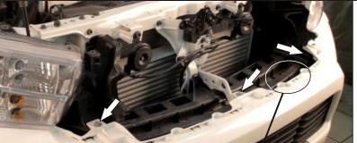
3. Remove upper bumper retaining screws and scrivets.
