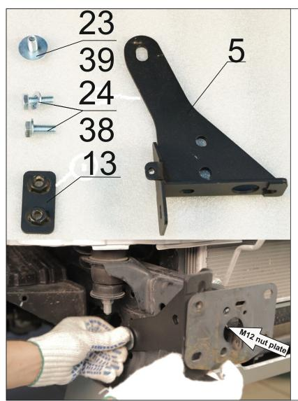
Winch bracket has been mounted to the Bumper Body for transport purposes.
