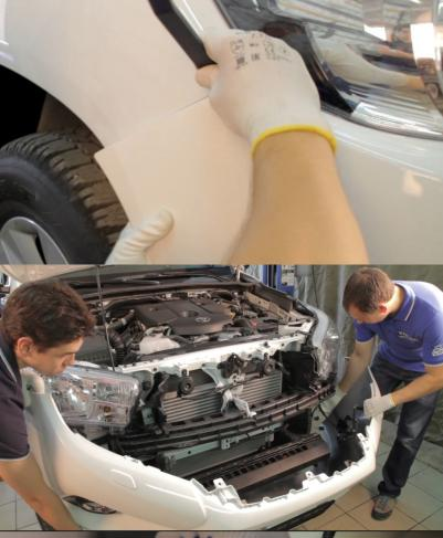
6. Carefully remove bumper from vehicle by pulling on each side of the bumper near the wheel arches and working your way towards the centre.
