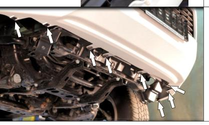
4. Remove lower bumper retaining screws.
