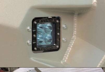
34. Install brackets with LED lights. Fix them with M6x16 round-head screws (26) and M6x12 washers.
