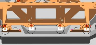
31. If there is a gap left between the winch bracket and adapter then insert the supplied adjustable plate of most appropriate size. Do the same for any gap between bumper body and winch bracket under the bolts of hawse. Tighten bolts after that.
