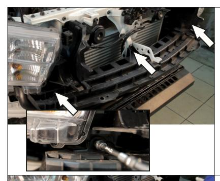
8. Remove 3xM6 screws from upper plastic deflector. Remove plastic deflector from vehicle and discard.
