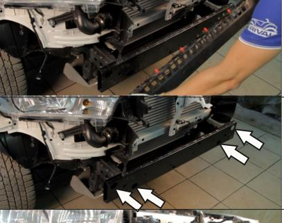
9. Forcefully pull the plastic crush absorber towards you and remove it.
