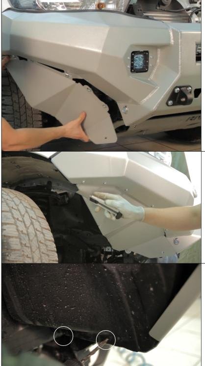
36. Install flaps using few M6x20 round-head screws and M6x12 washers.
