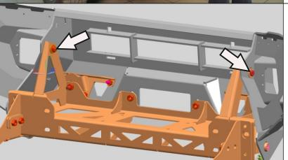
25. Mount bumper body onto the winch bracket using M10x30 bolts (22), M10x30 washers (37) and M10 nuts (32).
