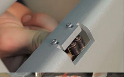
20. Mount roll latch (40) to bumper with screws M3x12 (25) and nuts M3 (30).
