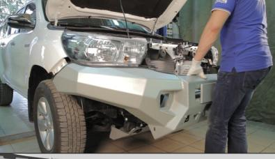
24. Install bumper body onto the winch bracket.
