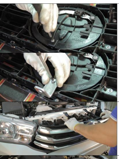
39. Remove lower screw out of radiator grill. Mount supplied bracket (17) using 4.2x16 screw (33) from fitting kit.
