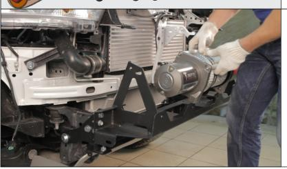
18. Mount the winch. Fix it to the mount with bolts supplied with the winch.
