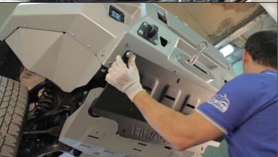
42. Install middle plate (10) between bumper and RIVAL skid plate. Fix it using 9x M10x30 countersunk-head screws (28) and countersunk washers (19).
