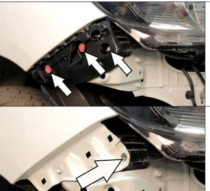
12. Remove M6 bolts and scrivets. Remove plastic side fittings.
