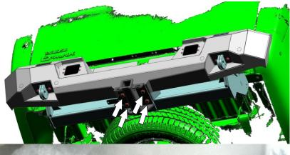
15. Install the tow bar (3) and socket bracket (M) to the bracket (2). Fix it using bolts M12x40 (B). Do not tighten yet. Adjust the bumper. Tighten bolts after that.
