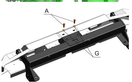
7. Unscrew bolts M12x1,25x40 (pos.A) and washers 12 (pos.G), preinstalled as travel hardware, in bumper bracket (pos.2) and aluminum bumper body (pos.1).
