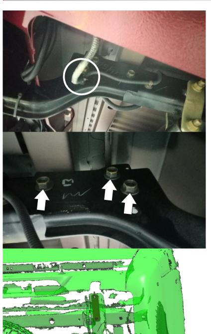
4. Remove wires and clips from the bumper
