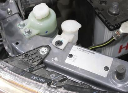
19. Remove the washer reservoir tank filler. Disconnect wiring from the washer reservoir. Dismantle the washer pump.
