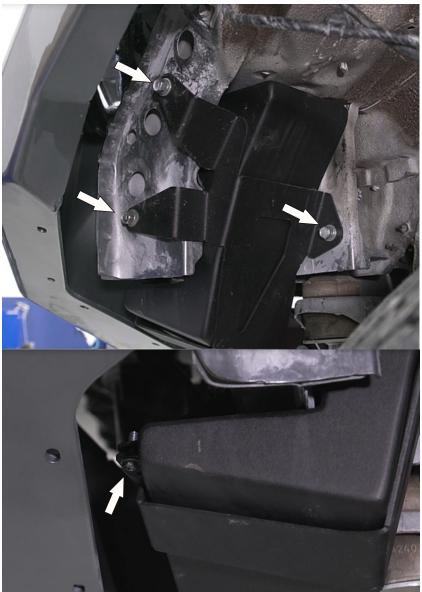
40. Install the washer reservoir (7) using the bracket (8) and standard fittings.
