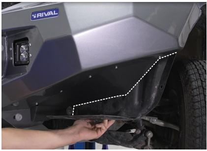
47. Install mudguards onto the vehicle and mark the cutting line.
