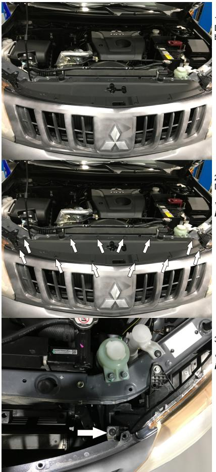
1. Open the hood. Disconnect terminal "-" from the vehicle battery.
