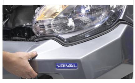
34. Adjust the bumper position in relation to the vehicle body. Where applicable, ensure even clearance of 15-22 mm. If required, move the bumper in cross direction, return to paragraph 29 and reposition adjustment shims.
