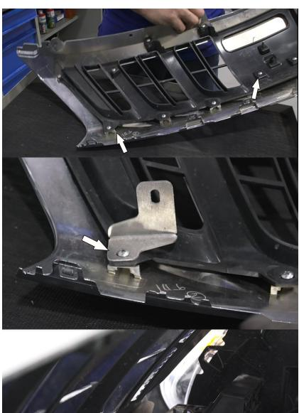
55. Unscrew specified screws on each side of the radiator grill.
