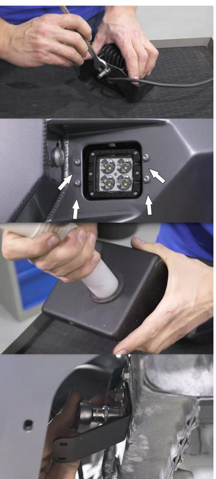
36. Install lights onto the brackets.
