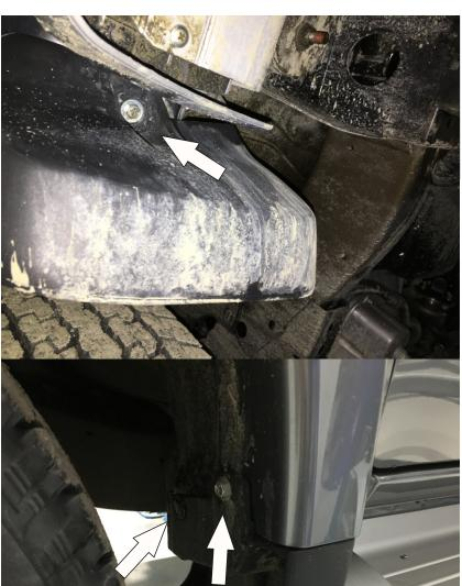
7. Unscrew the splash guard self-tapping screw
