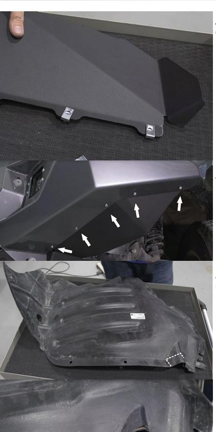
44. Install caged nuts (F) onto the flap (4, 5).
