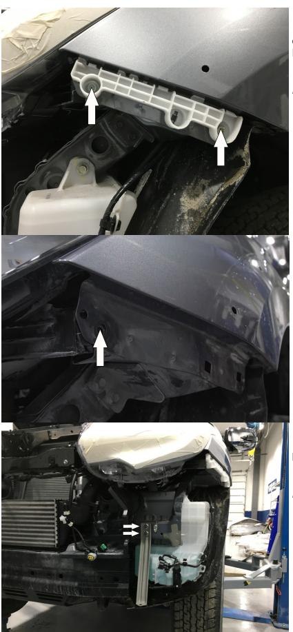
14. Unscrew bolt and self-tapping screw of the plastic clamper. Dismantle the clamp.
