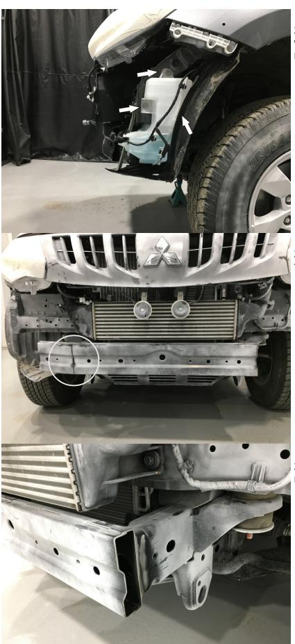
20. Unscrew 3 tension bolts of the washer reservoir. Dismantle the washer reservoir.
