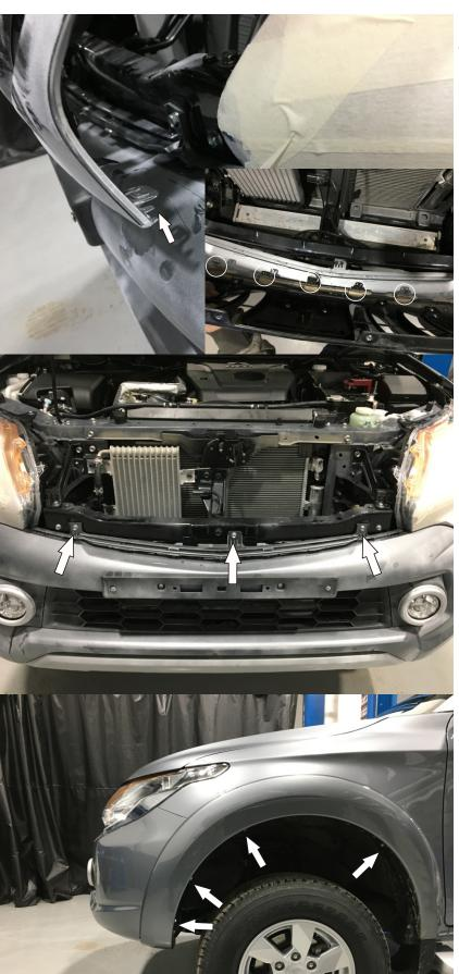
4. Dismantle the radiator grill. Carefully pull the grill edge by unlatching the latches.
