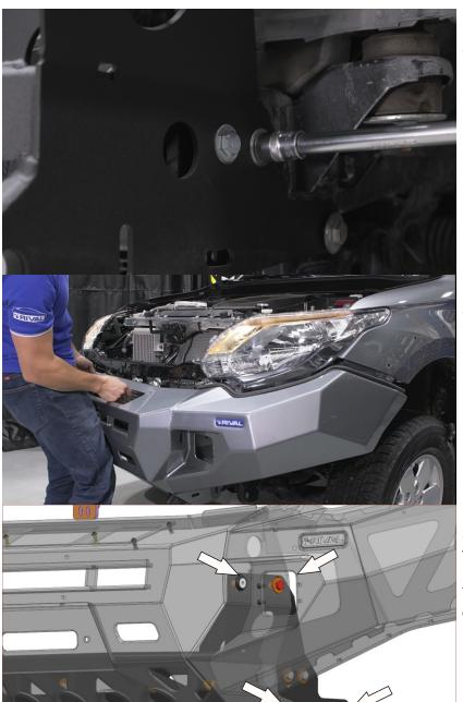
31. Tighten all screw joints of the bracket to the vehicle frame.
