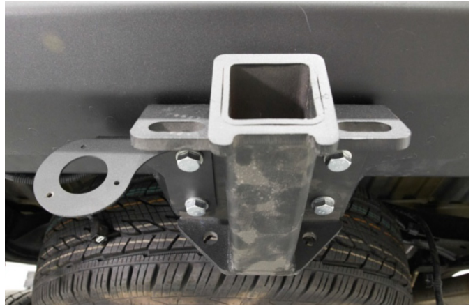
Fig. 18 18. Fix tow bar square (pos. 7) through tow bar socket bracket (pos. 12) using bolts M12x40 and washers 12 (pos. D,G). Tighten hardware after that.
