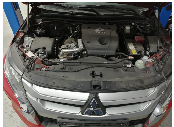
Fig. 22 22. Check all wires. Connect terminal “-” of the battery.
