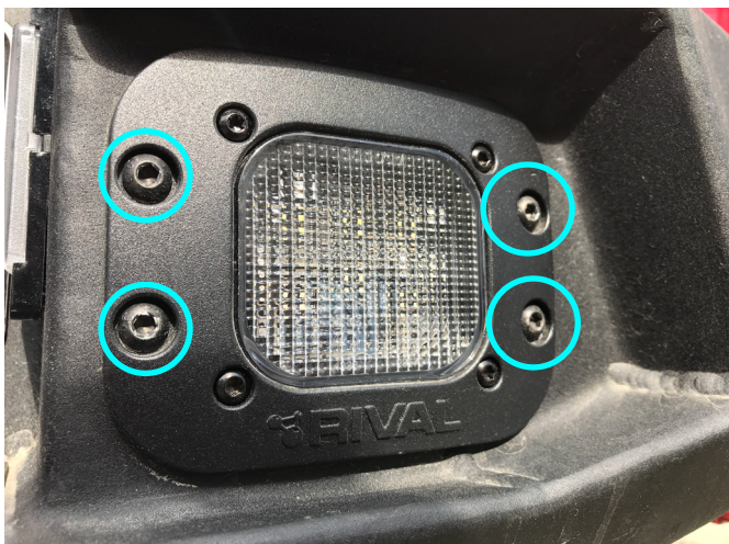
Fig. 21 21. Install LED lights or Lamp plug (pos. 11), using screw M6x20, Washer 6 and Nut M6 (pos. A, E, H).
