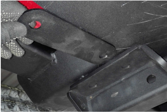
Fig. 17 17. Install adjusting plate (pos. 10) between bumper body (pos. 1) and tow bar square (pos. 7), as shown in fig. 17.
