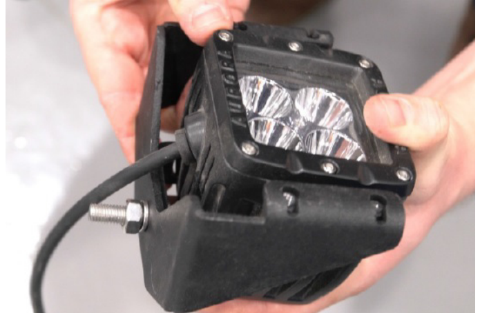
Fig. 20 20. Fix your aftermarket LED cudic lights to brackets (pos. 6). This brackets are not compatible with flush mount LED lights (parts number 2D.0042.1, purchused separately).
