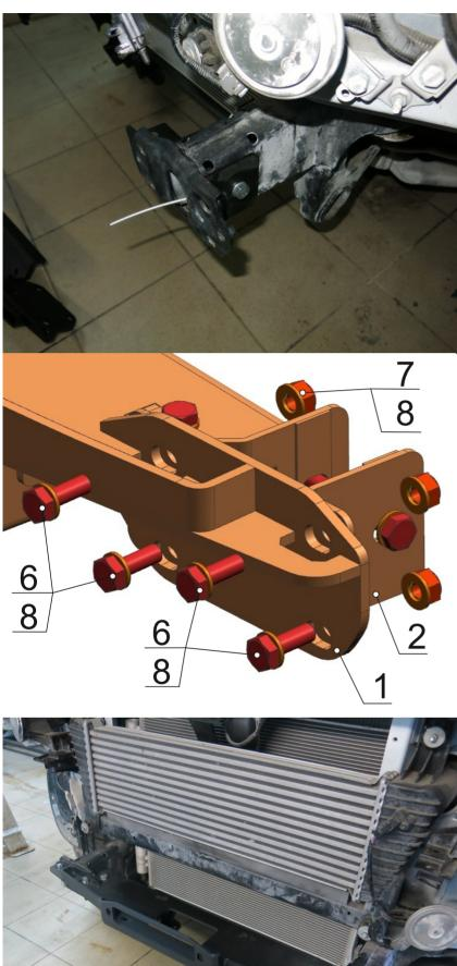
17. From outside of the chassis, mount outer bracket (2) from both left and right side. Fix them with bolts M10x30 (6), washers (8) to insert nuts (5).
