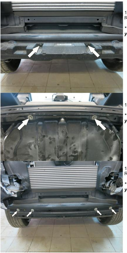
11. Remove the plugs out of the panel. Remove the panel.
