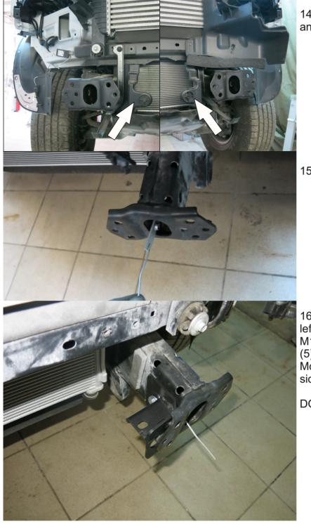
14. Remove plastic dusters from left and right sides of the vehicle.
