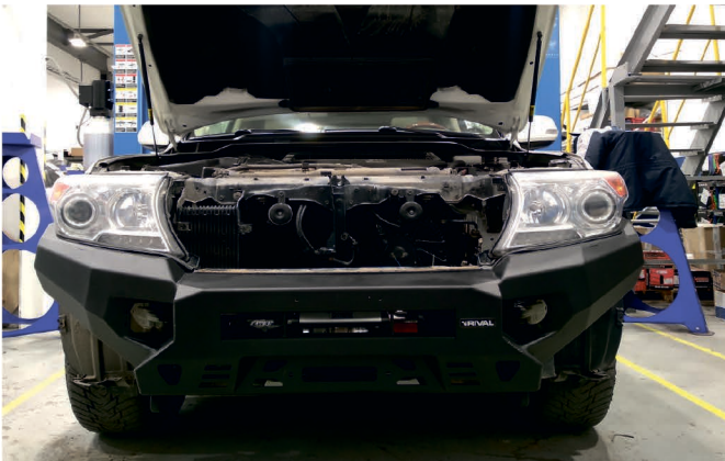
33. Install bumper body (pos. 1) onto the winch bracket (pos. 2).
