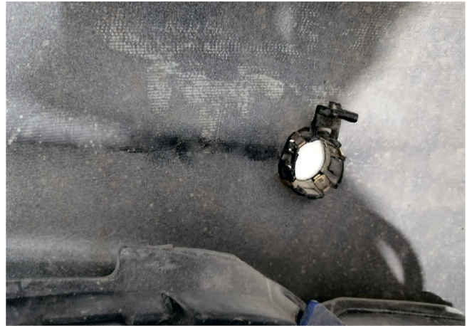
26. Remove parking sensors from factory bumper.
