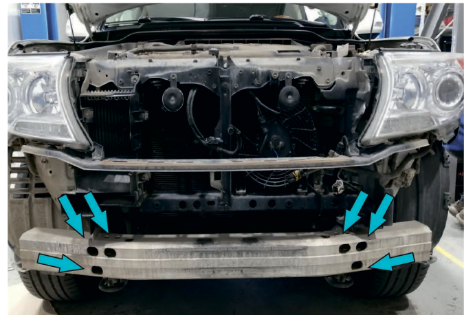
16. Remove damper. Unscrew 3 screws on each side and remove beam.
