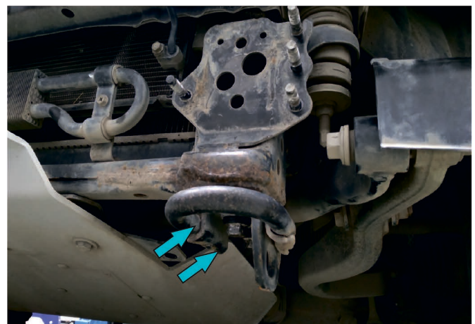
18. Unscrew 2 bolts and remove towing eye on each side.
