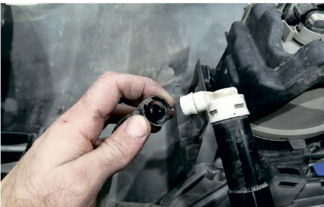
29. Disconnect the hose from the headlight washer.
