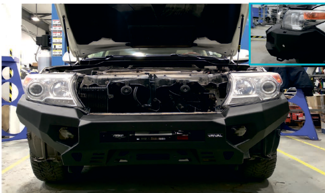
35. Align the bumper body with the vehicle. Tighten all the hardware.
