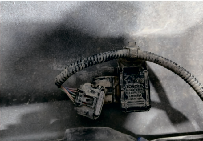
25. Disconnect the plug from the parking sensor.
