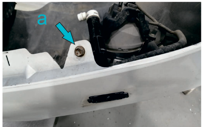
30. Unscrew the screw (a). Remove headlight washer.
