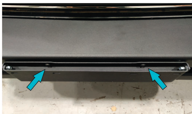
47. Attach license plate bracket (pos. 3) to bumper body, using bolt M6 (pos. B), penny washer 6 (pos. G) and nut M6 (pos. E).
