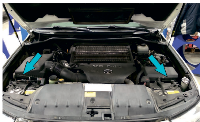
48. Connect all the wires and check it. Install plastic pad in reverse order. Connect terminal "-" of the battery.
