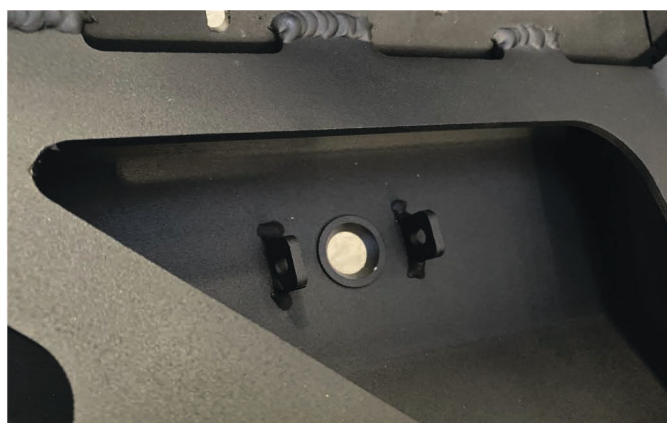
29. Install countersunk washer (pos. T)
