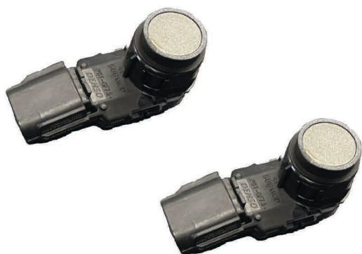
27. Remove parking sensors from factory bumper.
