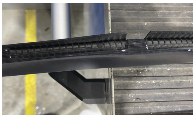
41. Remove the reinforced section of the seal.
